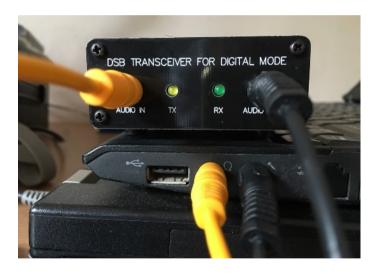
FOR LEGACY COMPUTERS WITH SEPARATED MIC AND HEADPHONE CONNECTORS, JUST CONNECT AUDIO IN TO HEADPHONE CONNECTOR, AND AUDIO OUT TO MIC CONNECTOR.
