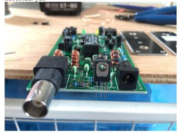
Put on the screw and nut for Q4, and put on nuts for BNC connector as well. Make sure the thermal pad is between the rear
