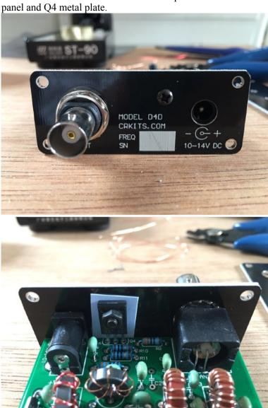
[ ] Align the DC IN connector hole, and turn over the board to make sure the board edge is in parallel with the rear panel edge, then solder. After soldering, fix the nuts tightly.
